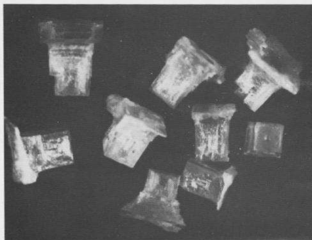
Fig. 11. Open and covered boxes of NaCl (magnification 3\times , 1\text{ cm} = 3\text{ mm} ).
