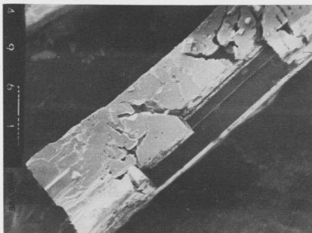
Fig. 2. Large inclusion with a 2 mm long salt crystal (segment).
