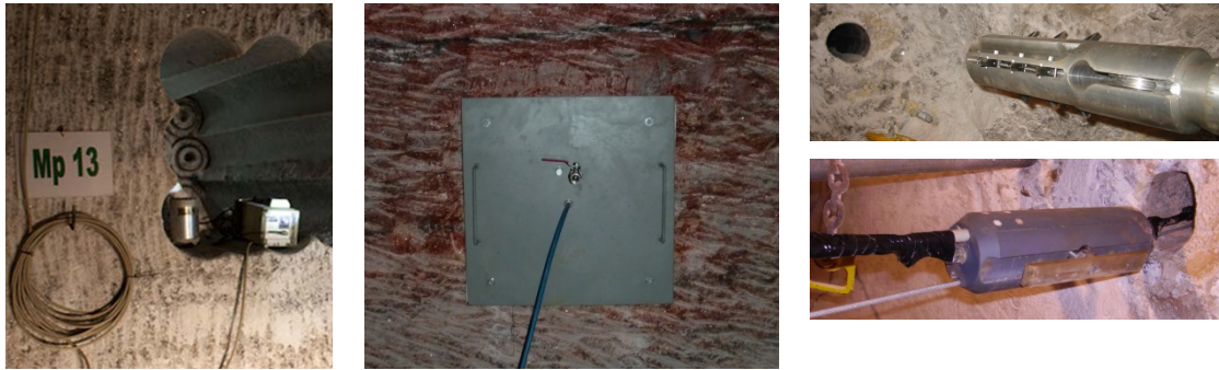
Figure 2: Examples for sensors and data transfer of underground seismic monitoring
