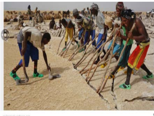
Figure 5. Levering up slabs of layered salt
